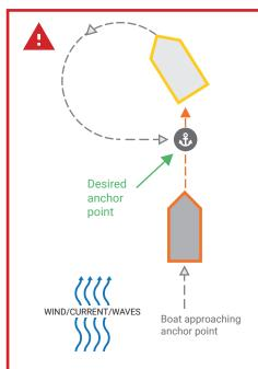
**CAUTION:** Setting anchor with wind/waves/current at your stern will cause the boat to overshoot and circle back to the anchor point and may result in motor cord wrapping.
